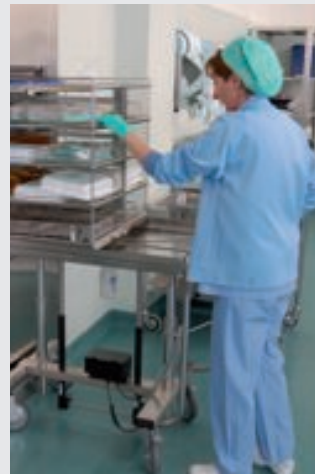
Automatic washing and disinfecting machines unloading side
