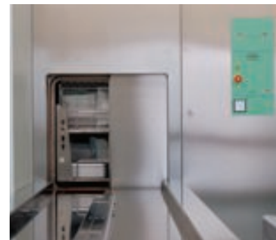
Automatic Steam Sterilizer load/unload system
